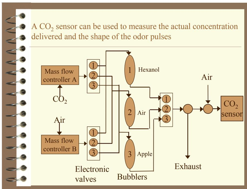
Figure 6.5. Using carbon dioxide as an odor tracer.
